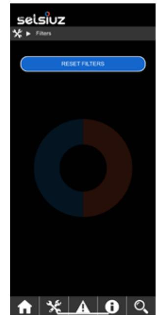
6. After having installed the filter in the Cooler, it can be reset here, so that you can keep track of exactly how long the filter has been in use in the overview.
